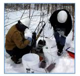
Groundwater samples were collected from four monitoring wells installed at the site. A specialized drill rig was used to create a deep, narrow hole in the ground (called a borehole), into which a monitoring well was assembled and placed into the drilled borehole. Groundwater
